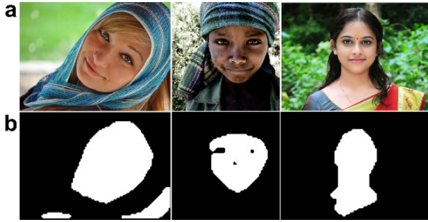
Fig. 3 (a) Three portrait images of people with different skin color and diverse background and luminance conditions, and (b) the output bitmap O_2 of the skin detection process.
