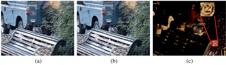
Fig. 23 a Original image. b Watermarked image. c Watermark readability with logarithmic-negative image processing. Test image 'outdoor' was obtained from UCID dataset
