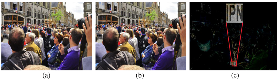
Fig. 21 a Original image. b Watermarked image. c Watermark readability with logarithmic-negative image processing. Test image ‘people’ was obtained from RAISE-1k dataset
